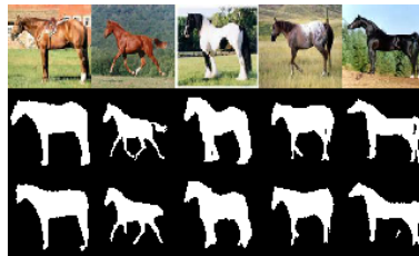
Figure 1. Sampled segmentation results. The top row contains the input images, the second row contains the ground truth masks, and the third row contains the c-Glow predictions.
